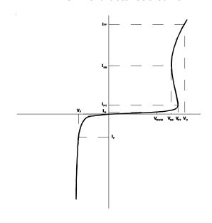
current ( $I_{SB}$ ). To return to a non-conducting state, the current through the device must fall below the  $I_{SB}$  (approximately <50mA) and the voltage must fall below the  $V_{SB}$  (normally 2.8 volts for a 3.3V device). If a 3.3V TVS is connected to 3.3V DC source, it will never fall below the snap-back voltage of 2.8V and will therefore stay in a conducting state.
