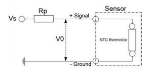
Vs = 5V  $\pm$  0.25V Rp = 2.21k $\Omega$   $\pm$  1% V0 = Measurement results based on RT curve
