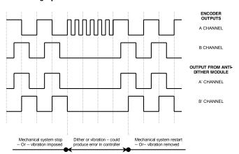
Note: For simplicity of illustration, the inverted channels, A/ and B/ have not been shown. The index, or Z, channel is also not shown in the associated diagram but is passed through directly as an optically isolated signal and maintains its original relationship to the encoder output channel. Reference Optical Isolator Module data sheet for connection diagrams.
