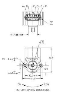
1 Connector mates with Packard Electric METRI-Pack 150.2 series (pull-to-seat 6 pin sealed connector assemblies) (i.e. 12162261, 12162260 or 12162210)
