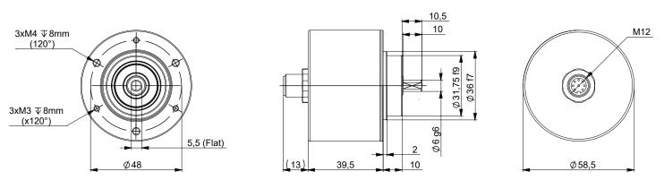
AH05\_14 Standard clamping, Connection BJR (Radial Cable)
