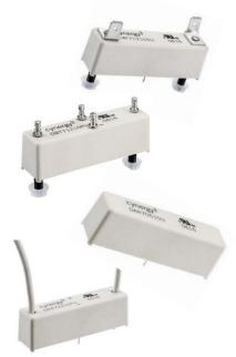
Recently approved by UL, very high isolation voltages (up to 10kV) are achieved through the use of high vacuum reed switches with either rhodium or tungsten contacts and make these relays suitable for high reliability applications, such as cardiac defibrillators, test equipment and high voltage power supplies.
