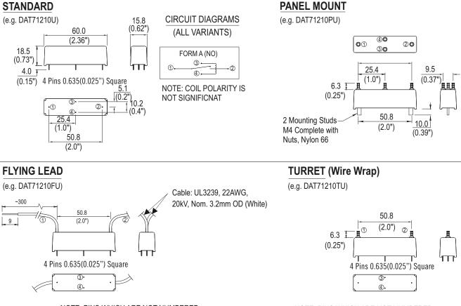
NOTE: PINS WHICH ARE NOT NUMBERED HAVE NO ELECTRICAL CONNECTION.
