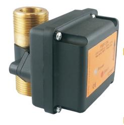
The FSV10AR can be used to control a pump or some other equipment or process via a relay output. If used in a pumped system, the device has to be fitted in the pipe above the pump.
