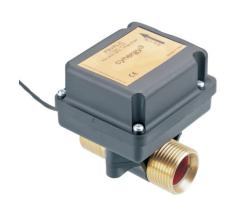
The FSVPLC can be used to control some other equipment or process via a PLC. If used in a pumped system, the device has to be fitted in the pipe above the pump.
