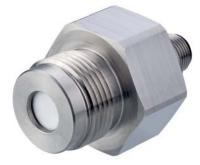
The semi-flush mount pressure transmitter, IPSS, has a piezo-resistive silicon or ceramic pressure sensor. The sensor is semi-flush to the housing making this product ideal for viscous or paste like media. The sensor and housing are made from stainless steel with a choice of internal '0' ring seals to ensure the product is suitable for a wide range of applications.
