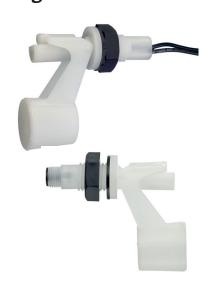
The RSF10 series drop float has been designed to eliminate problems associated with limescale build up around the pivot point of a conventional float switch. It is also suitable in more viscous liquids, that might affect the pivot action of a standard float type. This particular series is primarily for applications where a high level condition has
