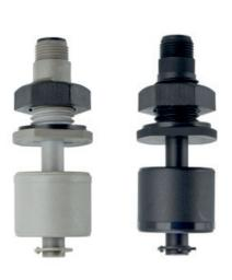
The RSF150 series are compact vertically mounted devices with a single switch point. Mounting is either from the top or bottom of a tank from the inside, so requires access to the inside of the tank.
