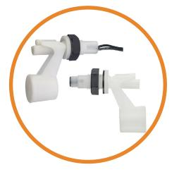
The RSF10 series drop float has been designed to eliminate problems associated with limescale build up around the pivot point of a conventional float switch. It is also suitable in more viscous liquids, that might affect the pivot action of a standard float type.
