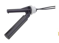
The RSF30 is a higher power side entry, internally fitted switch. These may be used for directly switching some small loads of less than 100VA. Fitting of this type requires access to the inside of the tank.
