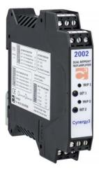
The SC2002ALM-HL trip amplifier can accept a wide range of user configurable inputs including 4-20mA, 0-20mA, 0-5V and 0-10V. The unit can have up to two relay outputs and each can operate as a high or a low trip; alternatively latching operation using both trip points can be configured.
