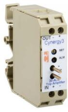
The SC20ALMDC is a 4-20mA direct current loop powered trip amplifier. The device derives its power from the input signal and therefore requires no external power supply. The output of the SC20ALMDC is a single pole, normally open, solid state relay which can be configured to close either above or below the adjustable setpoint. The switched output can be connected to any potential within 1kV of the transmitter supply, while transients of 2.5kV can be withstood.
