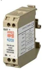
The SC420i loop powered isolator is a 0(4)-20mA direct current isolator. The isolator derives its power from the input signal and therefore requires no external power supply.
