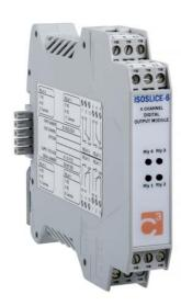
The SC-ISOSLICE-6 isolated Bus I/O module combines full three-port isolation with access to an industrial bus. This bus connects to the SC-E-100 modules which are then used to transmit the process values via either an Ethernet or a RS232/485 wired communications network.
