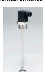
Top mount level switch with G1" (1"BSP) thread, enables this switch can be fitted to a tank through a G1" boss, without requiring access to the inside of the tank.
