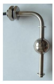
The SSV66-SM16 is a dual switch point side entry vertical float switch. This is mounted in a tank from the inside, so requires suitable access to the inside of the tank.
