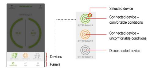
When the gadget logo (concentric circles) is green, it means that the environmental conditions measured by the gadget are deemed comfortable. If a device was connected during the runtime of the application but the connection is subsequently lost, the device logo will appear as grey in the list.
