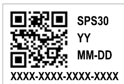
Figure 8: Label on SPS30
