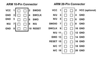
The 3V Pin of ST1 goes to VCC on the Debugger.
