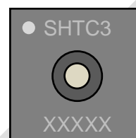
Figure 8 Laser marking on SHTC3, the top line with the pin-1 indicator and the sensor type, the bottom line with the 5-digit alphanumeric tracking code.
