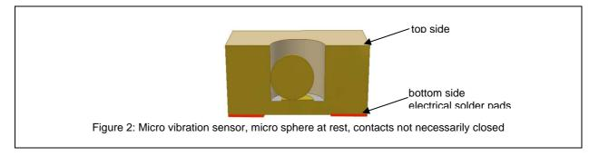
The unidirectional sensor version MVS1006.01 is open at rest, when mounted upside down position, so that the micro sphere is on the top side of the sensor, which has no contact.
