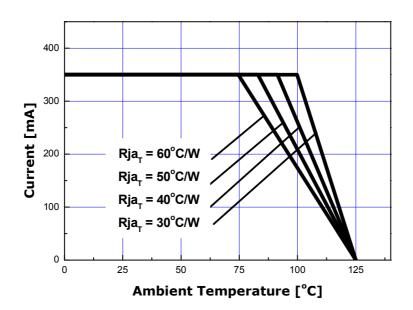
1-3. Photosynthetic Red (T<sub>JMAX</sub> = 125 °C, at 350mA)
