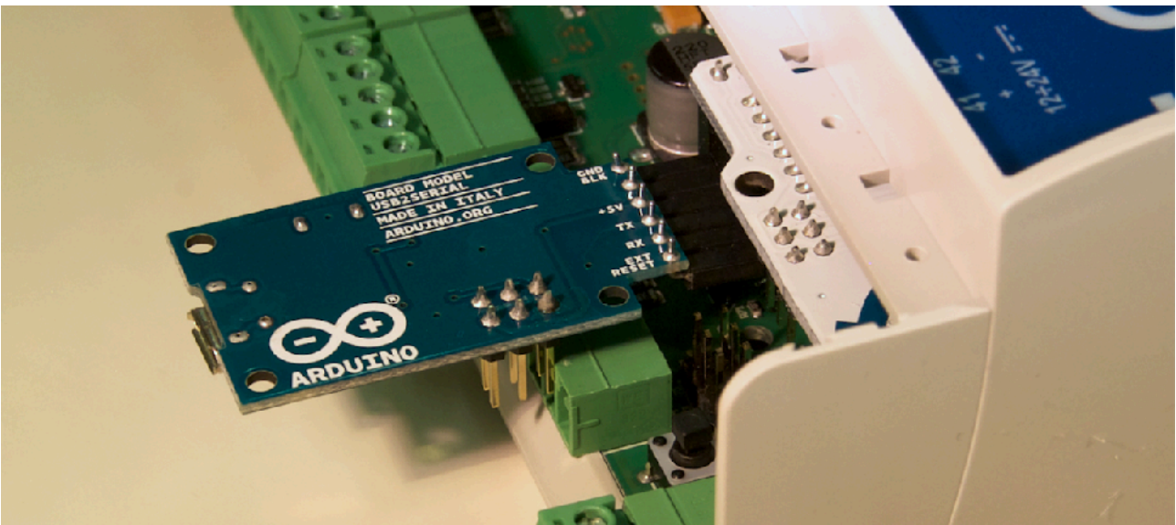
SERIAL ADAPTER CONNECTED TO THE ARDUINO BOARD
