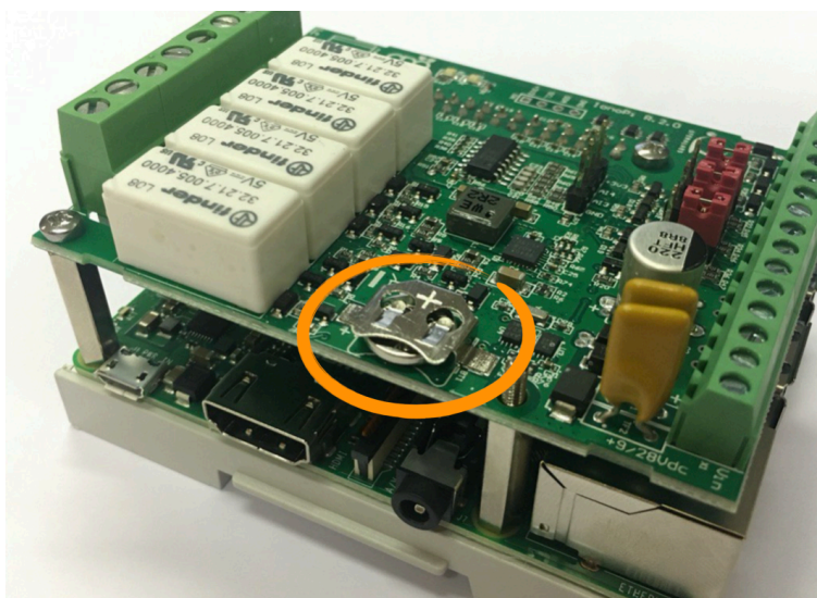
RTC BACKUP BATTERY
