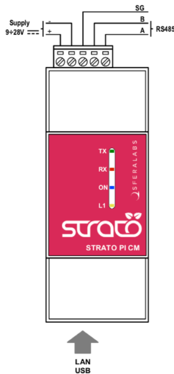
STRATO PI CM CONNECTION DIAGRAM
