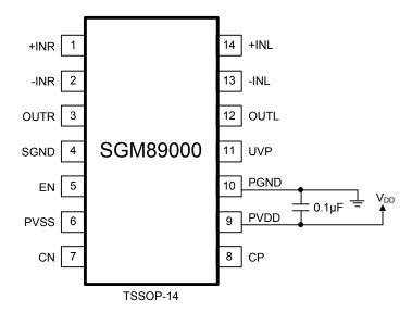
NOTE: 0.1µF decoupling capacitor must be close to PGND and PVDD pins; capacitor can be connected between PVDD and PGND pins directly and then connect PGND pin to GND layer.
