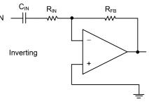
Figure 2. Inverting
