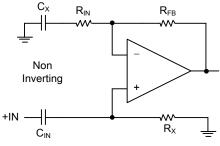
Figure 3. Non-Inverting
