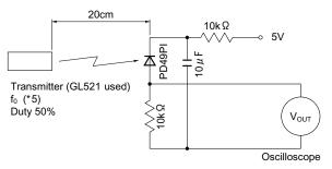
In the above figure, the transmitter should be set so that the output V<sub>OUT (P-P)</sub> can be 40mV. However, the PD49PI to be used here should be of the short-circuit current Isc=2.6  $\mu$  A at Ev =100 Ix. (E<sub>v</sub> is an illuminance by CIE standard light source A (tungsten lamp).)
