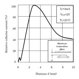
Fig.9 Relative Collector Current vs.
