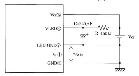
\*Note: LED-GND line and GND line must be separated.
