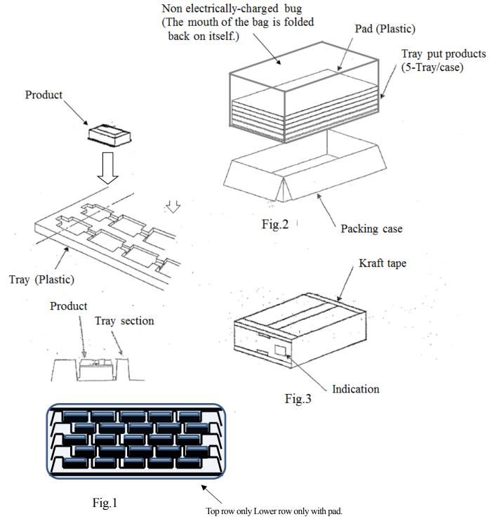
5 stacks (stack rotated by 180  $^{\circ}$  per stage. Inverted product storage direction)
