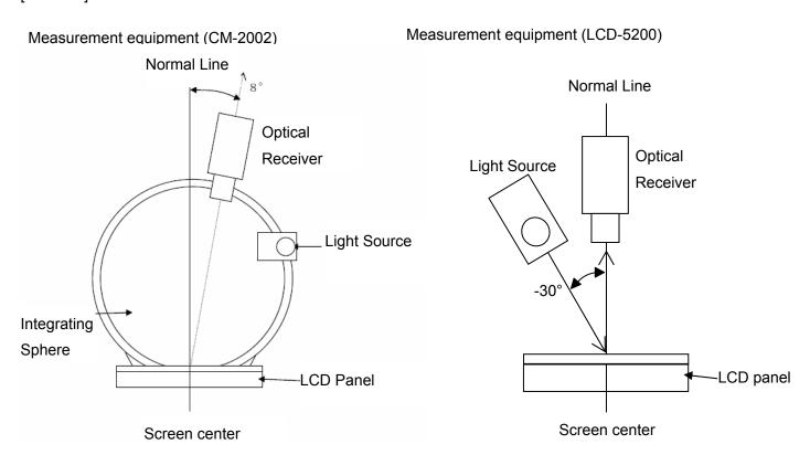
Figure 18 Measurement of contrast, reflective ratio and panel surface chromaticity
