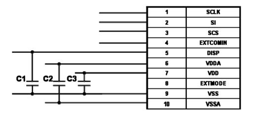
Figure 9-1 External circuit diagram (recommended)
