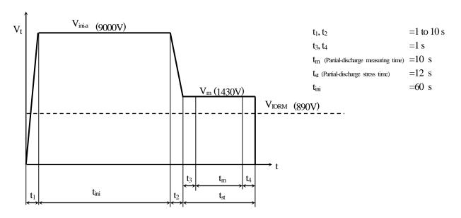
Method of Diagram 2: Non breakdown test (Apply to all device test)
