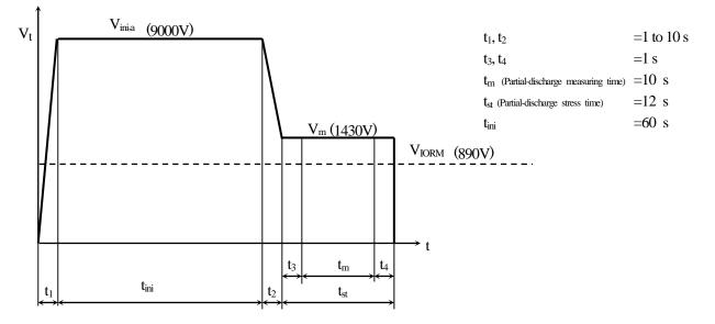
Method of Diagram 2: Non breakdown test (Apply to all device test)
