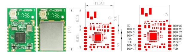
3-3: HY-40R204W / WMD40R204SR6W0( Metal WireAntenna)(1/4  $\lambda$  half wave dipole)\_
