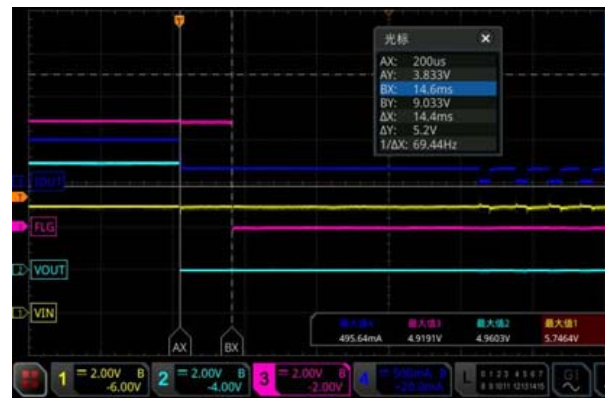
Output short circuit protection
