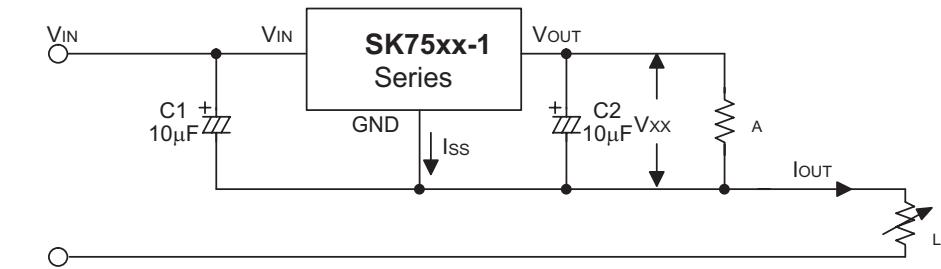
$$I_{OUT} = V_{XX}/R_A + I_{SS}$$
