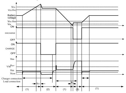
Figure 5-1 Overcharge and Overdischarge Voltage Detection
