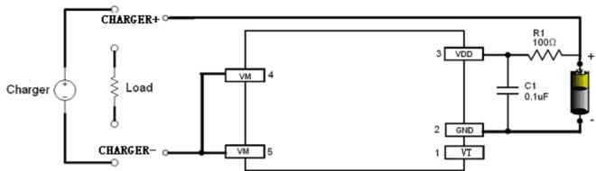
Fig 6 SD5351 in a Typical Battery Protection Circuit
