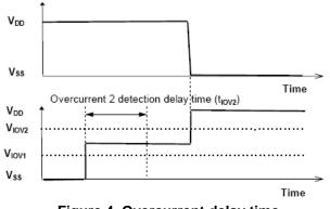
Figure 4. Overcurrent delay time
