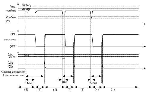
Figure 5-2 Overdischarge Current Detection
