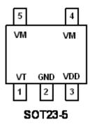
Figure 2. PIN Configuration
