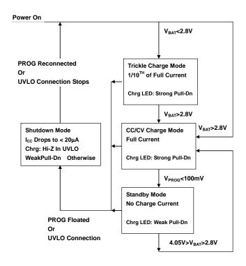
Figure 1. State Diagram of a Typical Charge Cycle
