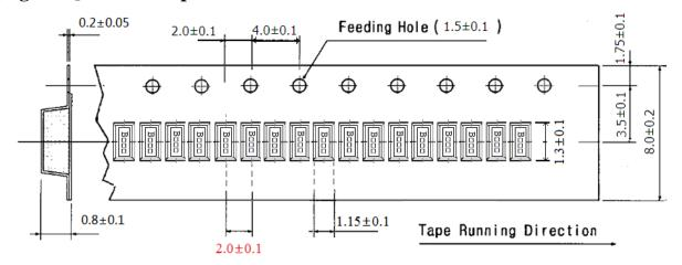
Prior to the size of  $4.0\pm0.1$ , after encryption, modified to  $2.0\pm0.1$ .
