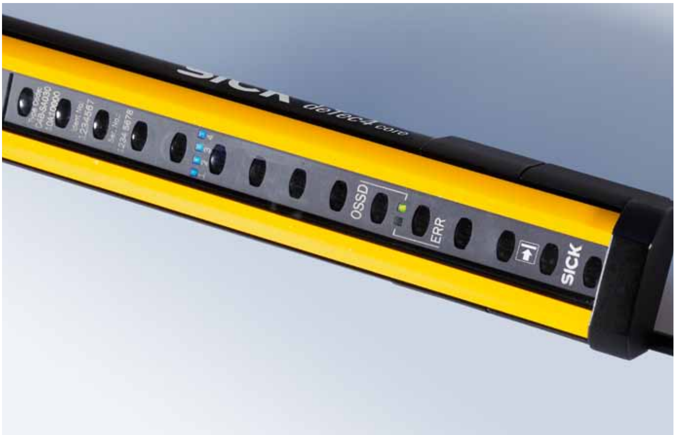
Direct feedback during alignment: the optimal position of the two housings relative to each other is indicated by the four blue LEDs.
