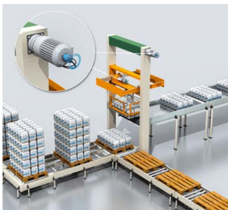
Palletizer system – positioning the gripper
