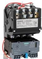
Non-reversing motor starter Size 1 Three phase full voltage Solid-state overload relay OLRelay amp range 3-12A 220-240/440-480VAC 60HZ coil Combination type No enclosure
