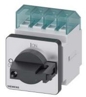
SENTRON, Switch disconnector 3LD, main switch, 4-pole, lu: 16 A, Operating power / at AC-23 A at 400 V: 7.5 kW, front-mounted, knob-operated mechanism, black, 4-hole mounting of the handle
