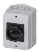
SENTRON, Switch disconnector 3LD, main switch, 3-pole, Iu: 25 A, Operating power / at AC-23 A at 400 V: 9.5 kW, molded-plastic encapsulation for inch cable gland, 1 NC, 1 NO, rotary operating mechanism, black
