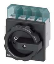
SENTRON, Switch disconnector 3LD, main switch, 4-pole, lu: 32 A, Operating power / at AC-23 A at 400 V: 11.5 kW, front-mounted, rotary operating mechanism, black, 4-hole mounting of the handle
