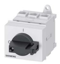
SENTRON, Switch disconnector 3LD, main switch, 3-pole, lu: 32 A, Operating power / at AC-23 A at 400 V: 11.5 kW, installation in distribution boards, knob-operated mechanism, black, handle direct at the switch
